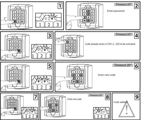
**WARNING:** To add a code, you need to know the system password. Q.BO TOUCH can handle up to 100 different codes. The new code will serve the same purpose as the existing code (activates the same channel).
